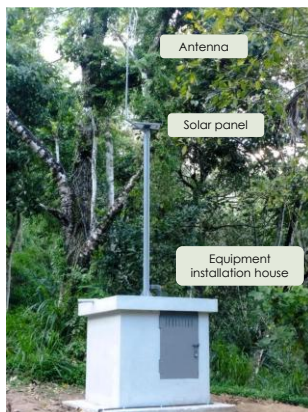
The River Water Level Sensor Station and the construction team after its completion in the APT Sri Lanka Smart Village Project
